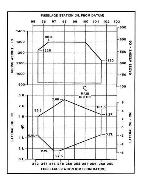
R22 STANDARD AND HP CENTER OF GRAVITY LIMITS
