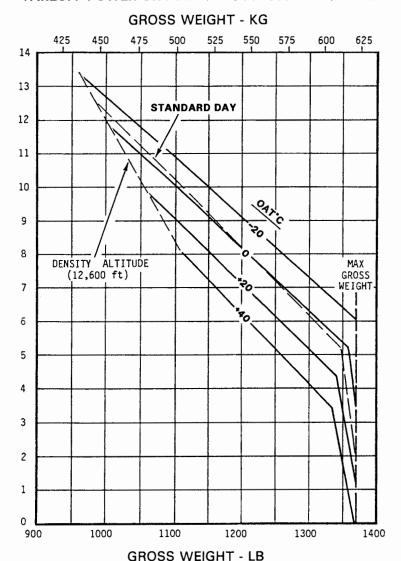
**R22 MARINER** 0-320-B2C Engine 5 Minute Takeoff Rating **OGE HOVER CEILING VS. GROSS WEIGHT**
