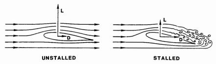
Wing or rotor blade unstalled and stalled.
