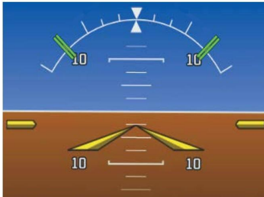
Figure S01-8 – ESP Roll angle limits
