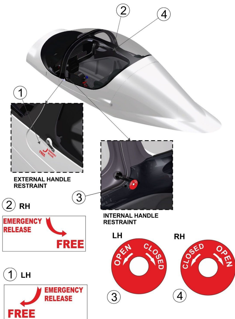
Figure 7-38 – Emergency Exit Placard
